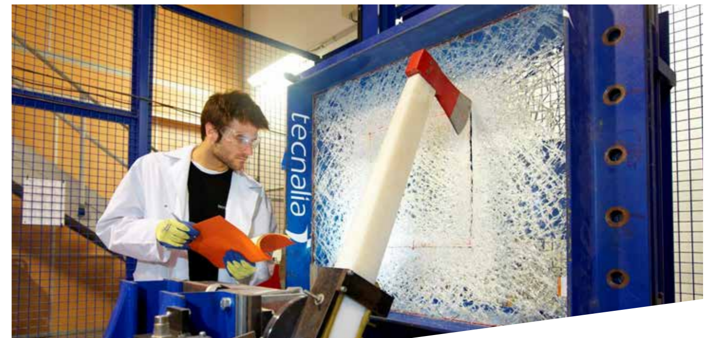
Simulation of the impact of concentrated load
